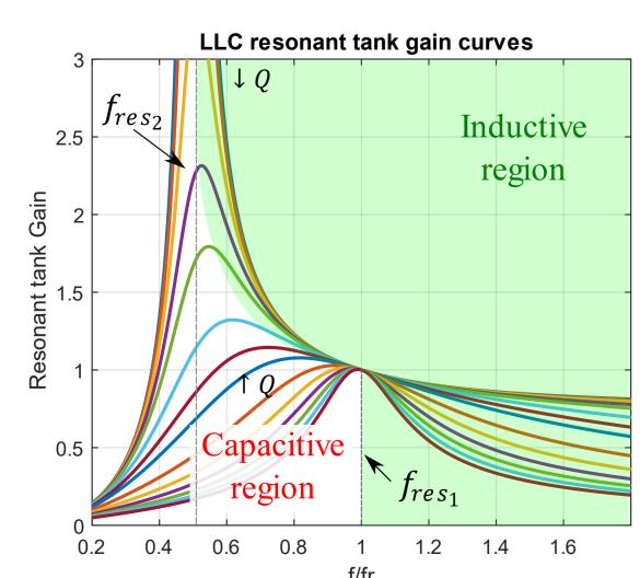
$$m = \frac{L_r + L_m}{L_r} \quad Q = \frac{\sqrt{L_r/C_r}}{R_{ac}} \quad F_x = \frac{f}{f_{res}}$$
